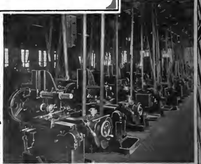
C—Battery of Brown & Sharpe Gear-cutting Machines Indicating Something of the Requirements from the Point of View of Quality and Quantity of the Gears Turned Out
